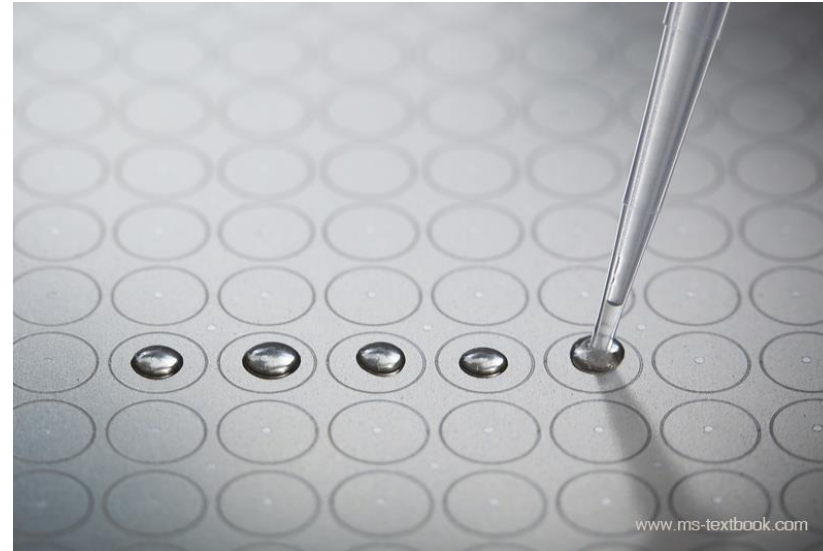
Manual spotting (Sample is mixed with matrix and applied to the metal plate)
